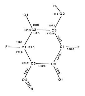
Fig. 1. The molecular structure of fluoranilic acid.
